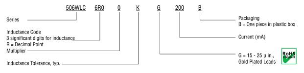
The above part number refers to a 506WLC Series 6.0 µH inductor, K tolerance (±10%, typ.), with Gold Plated Leads (G), 200 mA, one piece in plastic box.
