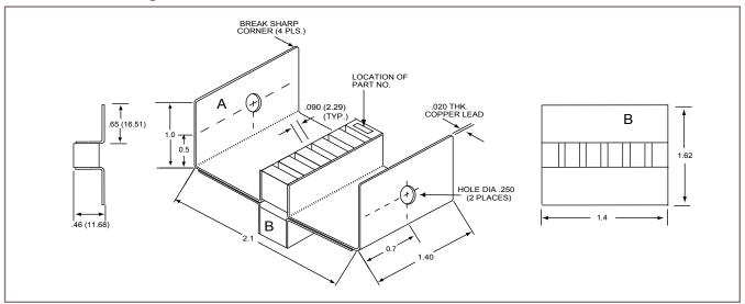
NOTES: The Assembly pictured above is constructed with 100E Series Capacitors.
