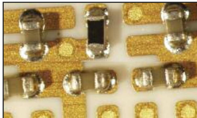
0201 Soldered to Filled Vias
